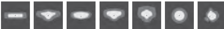
[T1] Type I, Asymmetric, Side throw [T2] Type II, Asymmetric, Side throw (AFX) [T2] Asymmetric, Side throw (ML) [T3] Type III, Asymmetric, Side throw [T4] Type IV, Asymmetric, Forward throw [T5] Type V, Symmetric [P4] Special pedestrian road distribution-right side traffic
