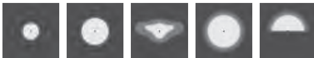
[S] Spot [N] Narrow [T2] Type II, Asymmetric, Side throw [SYM] Symmetric [ASYM] Asymmetric
