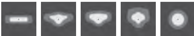
[T1] Type I, Asymmetric, Side throw [T2] Type II, Asymmetric, Side throw [T3] Type III, Asymmetric, Side throw [T4] Type IV, Asymmetric, Forward throw [T5] Type V, Symmetric
