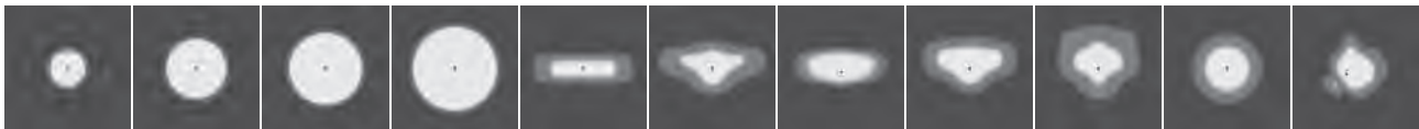
[S] Spot [N] Narrow [MN] Medium narrow [M] Medium [T1] Type I, Asymmetric, Side throw [T2] Type II, Asymmetric, Side throw (AFX) [T2] Asymmetric, Side throw (ML) [T3] Type III, Asymmetric, Side throw [T4] Type IV, Asymmetric, Forward throw [T5] Type V, Symmetric [P4] Special pedestrian road distribution-right side traffic
