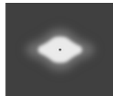
[T-SYM-D] Tunnel, Symmetric, Type D -
