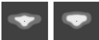
[T2] Type II, Asymmetric, Side throw - 137x52° [T3] Type III, Asymmetric, Side throw - 143x68°
