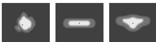
[P4] Pedestrian crosswalk distribution - 20x78° [T1] Type I - 111x48° [T2] Type II - 133x48°
