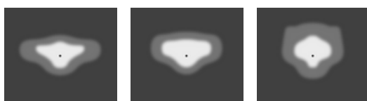
[T2-2] Type II - 149x54° [T3] Type III - 143x63° [T4] Type IV - 117x64°
